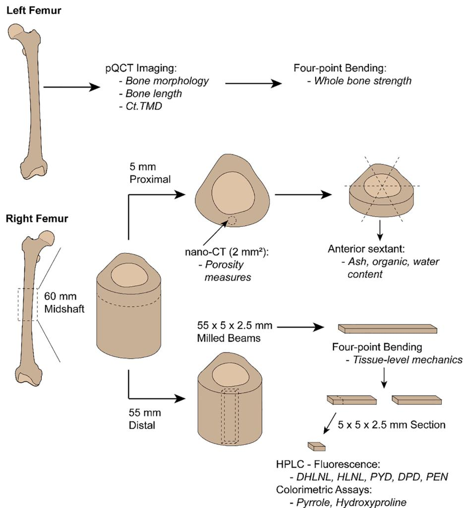
**Fig. 1.** Distribution of tissue from left and right femora for each characterization method. Output(s) from each characterization technique are italicized. Milled beams and cut sections are presented as L × W × H. Not drawn to scale.
