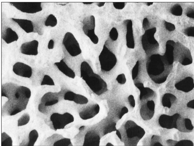
Fig 23-11 Porous coralline hydroxyapatite ceramic augmentation material (Pro Osteon Implant 500, Interpore Cross International).
